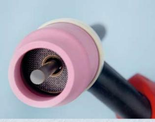
In water-cooled welding torches, the cooling ducts extend around the underside of the gas nozzle. This gives the weld process additional stabilisation.
