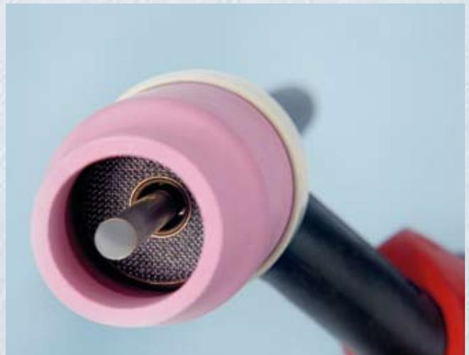
*Using the shielding-gas lens ensures high weld-seam quality at the same time as saving as much as 20 % of the shielding gas.*
