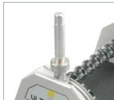
Tip may be flattened by 1/10 mm per point in the 90° position.
