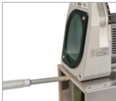
Precise adjustment of the electrode's stick-out.
